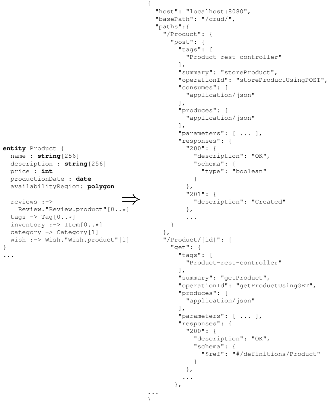
Figure 1: TyphonML model and corresponding OpenAPI specification generated from it (extracts)
